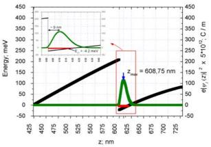
Fig. 3. Quantum well formed at the GaAs/AlGaAs interface (black line and left axis). Energy of the ground state  $E_{z1}$  (red line) and corresponding wave function  $\psi_1(z)$  (green line and right axis). The inset shows the neighbourhood of the heterojunction.
