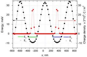
Fig. 5. Cross-sections of charge density (red circles) and potential distribution (black squares) after self-consistent procedure, performed in xy plane. There are also energy levels  $E_0$ ,  $E_1$  marked in each quantum well.
